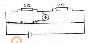
The diagram above illustrates a metre bridge circuit under balanced condition.
